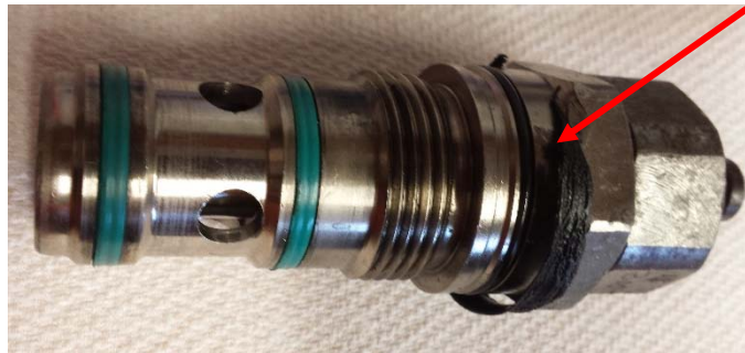
Failed Back-up Seal
