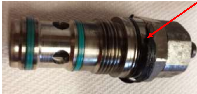
Failed Back-up Seal
