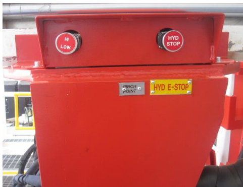
Hi – Low and hyd E-stop valves fitted to turret
